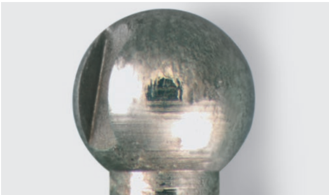
Damage caused by a plastic female part: Irreparable damage to the male part caused by a build-up of substances in the plastic
