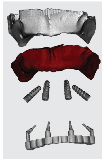
Figure 1: Components of the FE model used in this study. The model of the bone is based on a CT scan, while the surface of the mucosa is based on an optical scan of a plaster cast of the same case. Implants were modelled from CAD data, and the idealised bridge was modelled manually.
