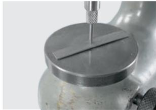
**Measurement of deformation:** After simulation of ceramic firing cycles
